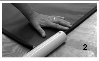
Insert fabric sleeves into the channel on each length of pipe.
