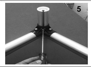
Place rubber caps on legs and insert legs into bottom corner. Rotate leg so slot aligns with set screw hole. Secure in place with set screw. This is purposely a tight fit so it will take some effort to fully tighten screws. Turn bed over and fully tighten all screws and nuts so they are flush with the nylon insert locking material.
