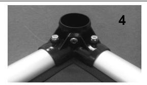
Place a bottom corner bracket over pipes, insert screws through openings, secure with a lock nut and hand tighten. Insert and secure second screw. Repeat process at each of other three corners.
