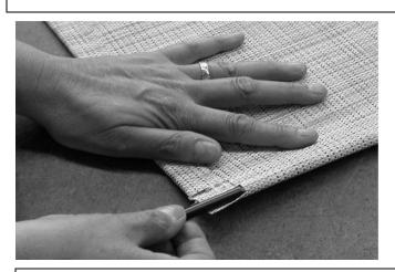
Lay fabric flat with underside facing up and insert cording into sleeve. Note that 40oz Vinyl fabric comes with cording in the sleeve.
