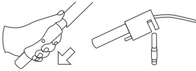
**2.** Remove the protective rubber from the pole head.
