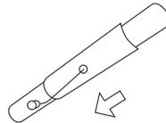
**6.** Disassemble the pole head by unscrewing it from the pole.
