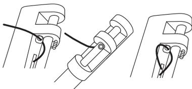
**17.** Tighten the pole head locking hex screw with a M2 size hex wrench. Replace the protective rubber onto the pole head.
