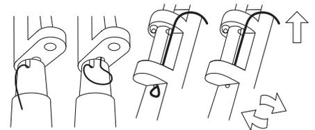
**16.** Insert the quick release cable through the end of hex screw. Pull the cable tight and then tighten the hex screw with a M2.5 size hex wrench. Tug the end of cable into the pole head cavity.
