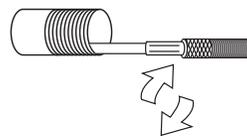
**12.** Re-insert the quick release cable until it is visible at the head of pole.
