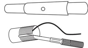
**13.** Wedge the quick release cable at the groove. The groove is located at the head of pole.
