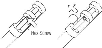
**5.** Pull out instant release cable by the copper end-nut, about 1 1/2 to 2 inch for enough clearance to disassemble the pole head.
