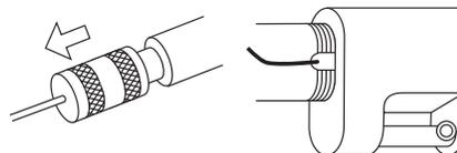
**15.** Tighten the pole head and then reverse about 1/8 of turn. Insert the instant release cable into the pole head and pull through the other end as much as possible. Continue the cable pulling and tighten the pole head.
