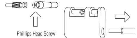
**10.** Insert the replacement cable from the noose end through the pole head. Once inserted, mount the Phillips head screw on the cable end, and tighten it.
